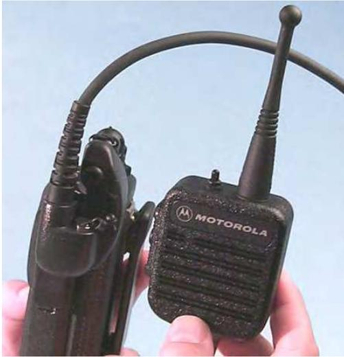
4. Attach the correct (frequency-sensitive) antenna to the PSSM by screwing the antenna's threaded end into the threaded antenna jack on top of the PSSM's housing.
