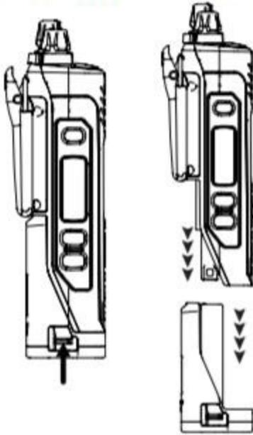
1. Push in the release tabs on each side of the battery.
